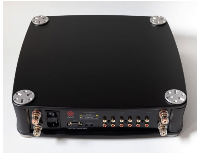
The rear panel of the I-280. All new Aavik amplifiers have the same connectors: 5x line In, 1x pre out, plus speaker terminals, which were sensibly placed quite far out (Photo: F. Borowski)
