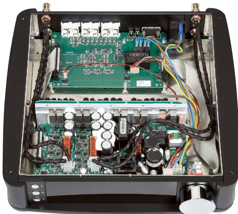
The internal construction is separated into input stage and power stage/PSU. The cables to the speaker terminals are from Aavik.
