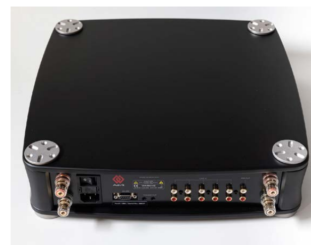
The connections of the I-580 correspond to those of the I-280 shown here: 5x line in, 1x pre out, plus speaker terminals, which were sensibly placed quite far out (Photo: F. Borowski).
