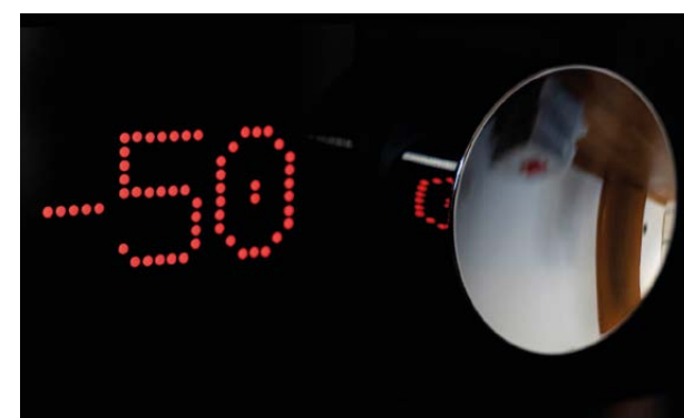
A close-up view of the red LED matrix display and the chrome-plated concave level control (Photo: F. Borowski).
