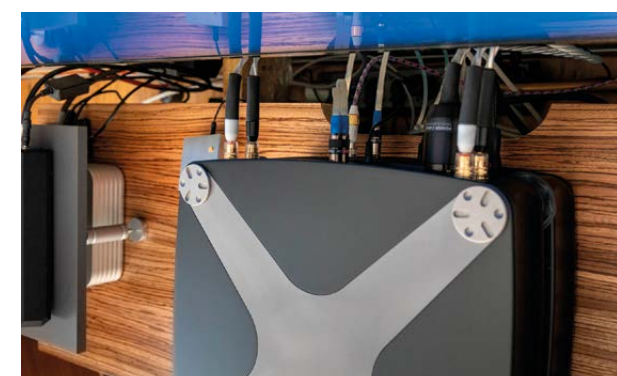
The loudspeaker terminals are located far out and thus do not come into conflict with the interconnects (Photo: F. Borowski)
