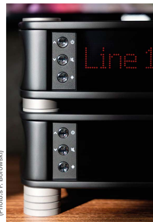
The optional Darkz device feet - shown here in the titanium version under the DAC - are used for „mechanical grounding“ and are surprisingly effective. The amplifier (above) is separated from the DAC here only by titanium balls. These lie in the recesses of the adapter pieces and ensure a stable and perfectly aligned stack
