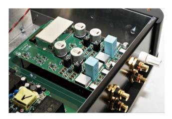
According to the manufacturer, the more coils are used, the more significant is the noise suppression, and the smoother the signal transmission, which results in quieter backgrounds, more clarity and a more vibrant sound in the audio replay.
