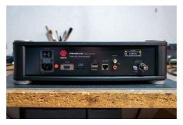
For the digital output, Aavik relies exclusively on SPDIF. A BNC and a Toslink connection are available for this. For external storage media, there are 2 USB ports and, of course, an Ethernet port. Obviously, nothing works without Ethernet!
