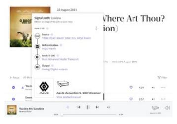
Signal path during playback of an MQA-encoded track from Tidal.
