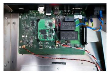
Streaming board, DAC and the power supply on the right: 2 encapsulated power supplies are used.
