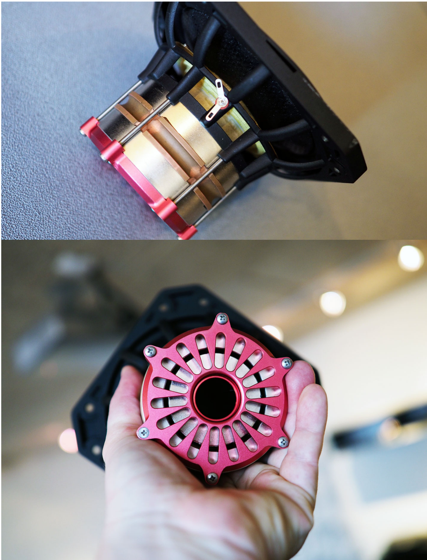
In the rear view it can be seen that the magnetic gap is completely open to the rear. This also reduces compression effects (Photo: Frank Borowski)
