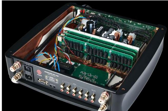
Here clearly visible, the inner copper chassis, and around it, the composite housing. Inside, among other things, the dither circuits and the Tesla coils of the top model Aavik I-580.
