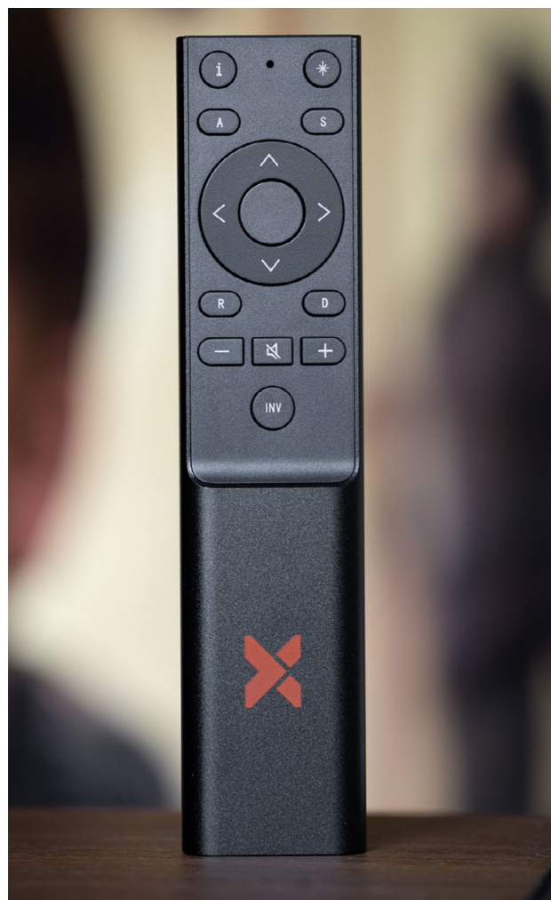
The corresponding IR remote control. However, it cannot be used for music control (play/pause, skip) during streaming (photo: F. Borowski)
